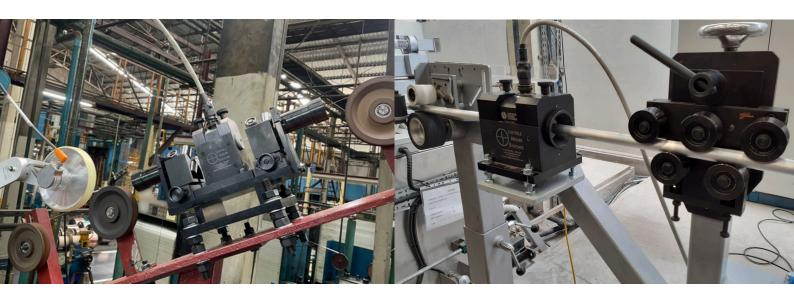
— Example of an Eddy Current coil support with guiding cones and pinch rolls
