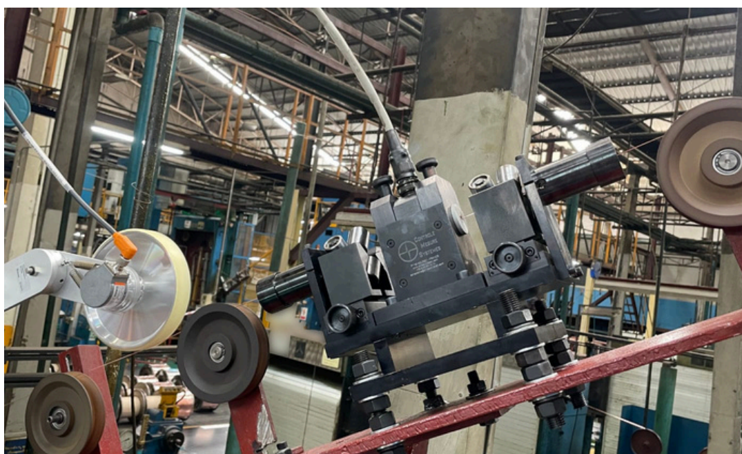
— Example of one of our CMS Eddy Current coil supports for aluminum and copper wire inspection
